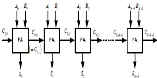
Fig. 1 N-bit Carry Ripple Adder
