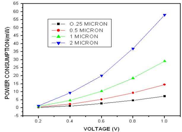
Fig.4: power consumption vs. applied voltage levels to the structure of Dilverp1 heater
