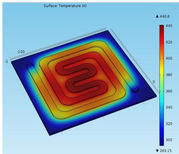
Fig1. Curved spiral heater over SiO<sub>2</sub> at 0.8V
