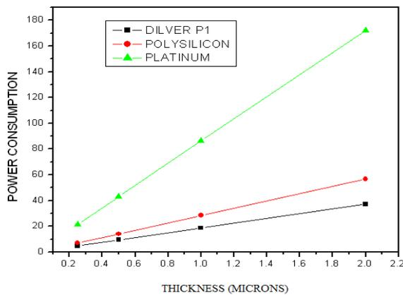
**Fig.5: power consumption vs. applied thicknesses Using different materials**
