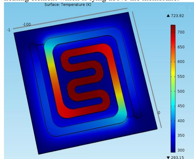
Fig 2. Curved Spiral heater with a cavity in the silicon at the center of micro-heater
