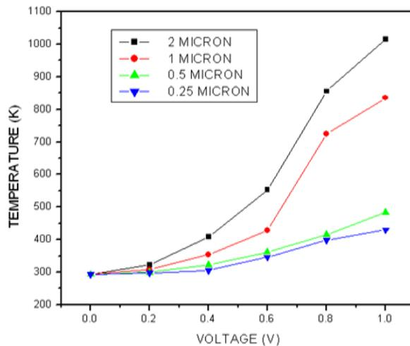
Fig.3: Heater Temperature vs. Applied voltage levels to the structure of Dilverp1 heater
