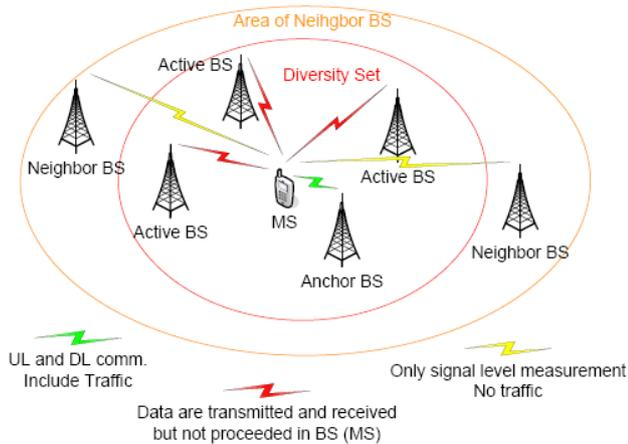
Figure 3. Fast base station switching[5].
