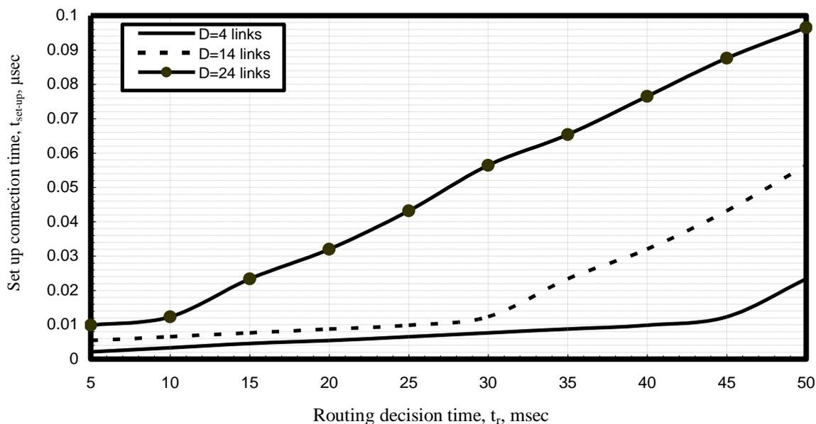
Fig. 1. Variations of set up connection time against variations of routing decision time and number of links at the assumed set of the operating parameters.
