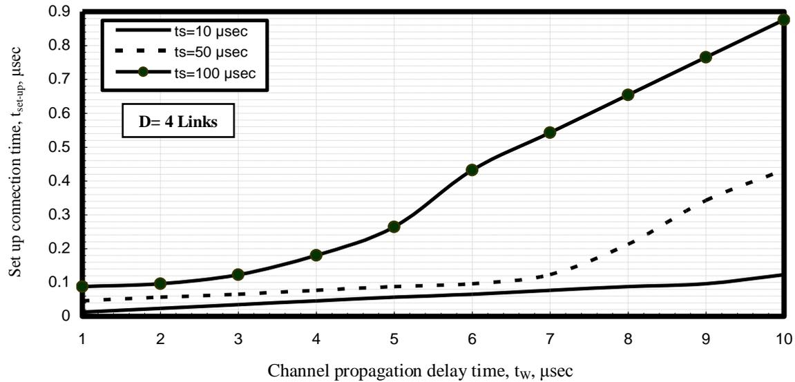
Fig. 2. Variations of set up connection time against variations of channel propagation delay time and switching delay time at the assumed set of the operating parameters.
