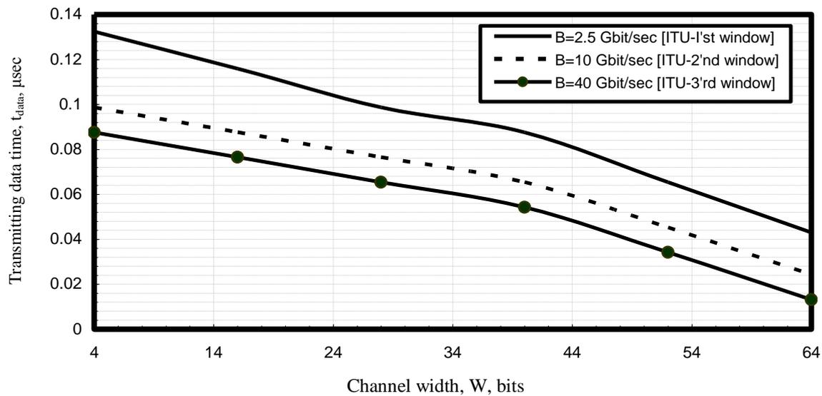
Fig. 6. Transmitting data time in relation to physical channel width and channel bit rate at the assumed set of the operating parameters.
