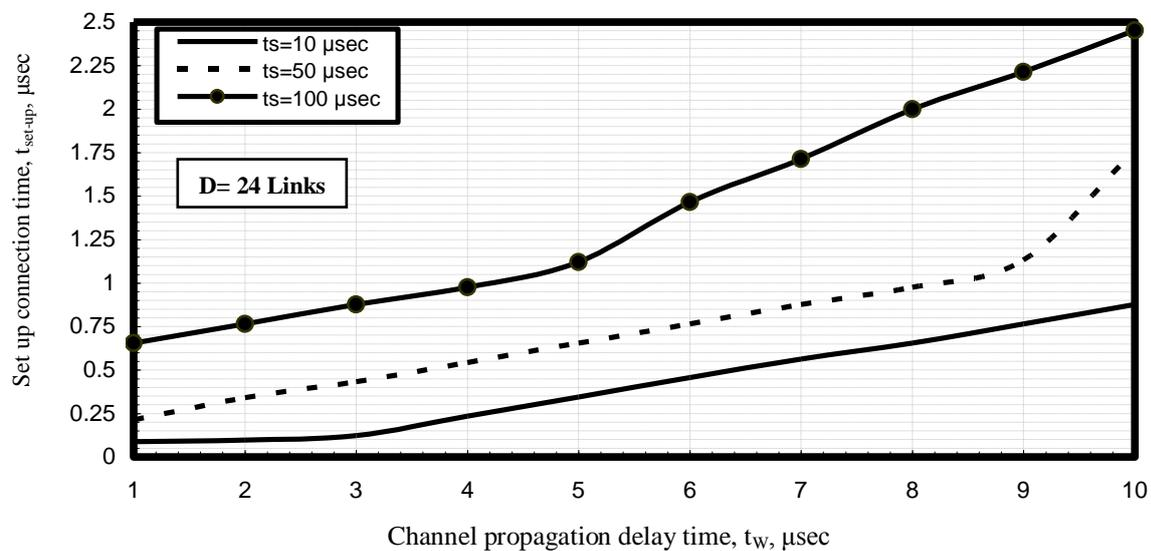
Fig. 4. Variations of set up connection time against variations of channel propagation delay time and switching delay time at the assumed set of the operating parameters.
