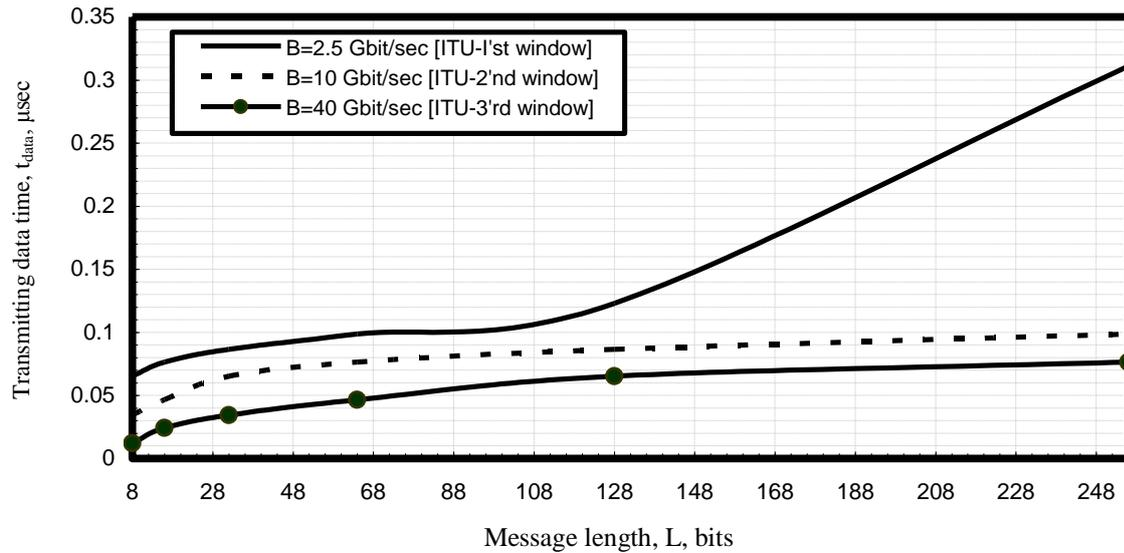
Fig. 5. Transmitting data time in relation to message length and channel bit rate at the assumed set of the operating parameters.
