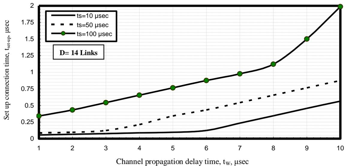
Fig. 3. Variations of set up connection time against variations of channel propagation delay time and switching delay time at the assumed set of the operating parameters.
