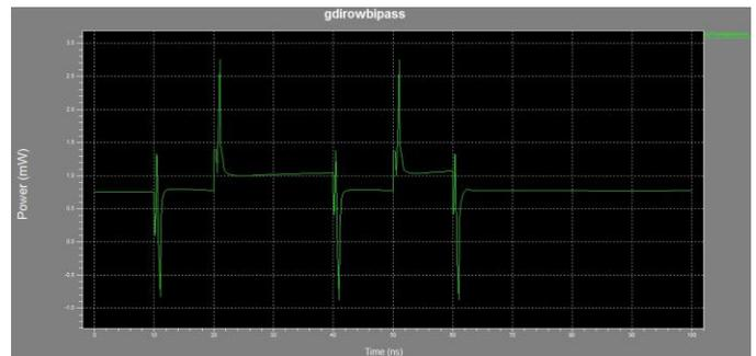
Fig 5.2: power consumption waveform of row bypass multiplier in GDI method
