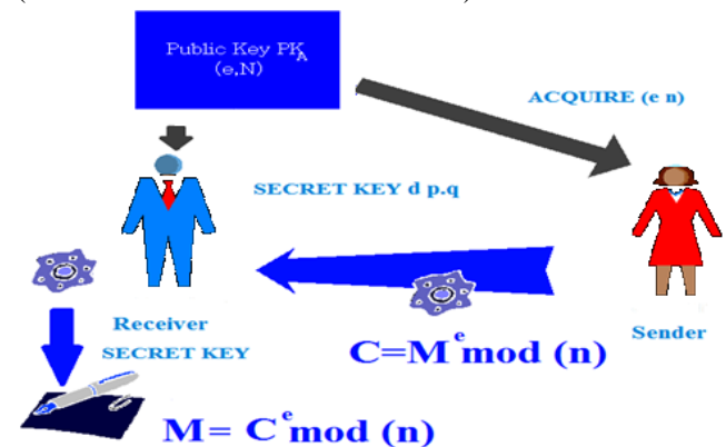
Figure 2 Basic working of RSA System
