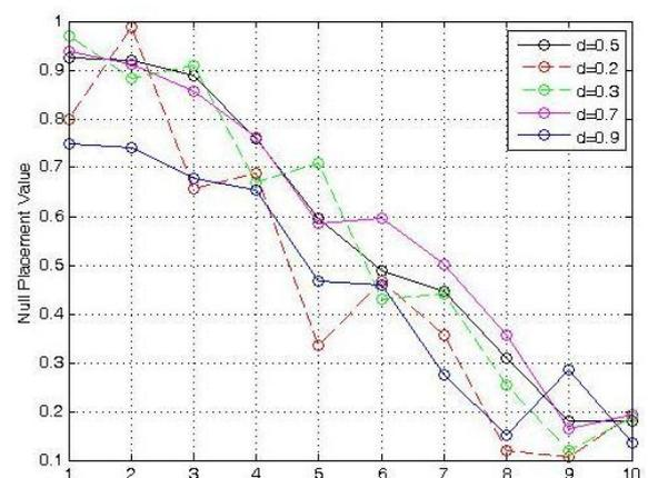
Fig. 10 NULL placement values after optimizing (1) for varying element spaces for d = 0.5, 0.2, 0.3, 0.7, 0.9
