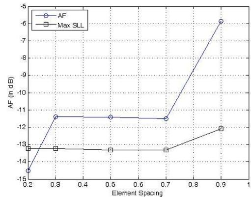
Fig. 9 Array Factor value with respect to the maximum sidelobe level value for element spacing 0.2, 0.3, 0.5, 0.7, 0.9.
