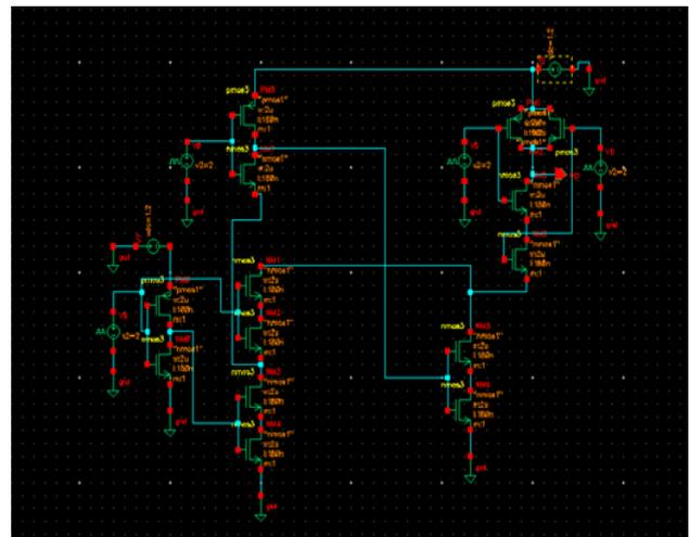
**Fig 5 Schematic Design of Hybrid MTCMOS Partial Stack Technique using tri-modal switch**
