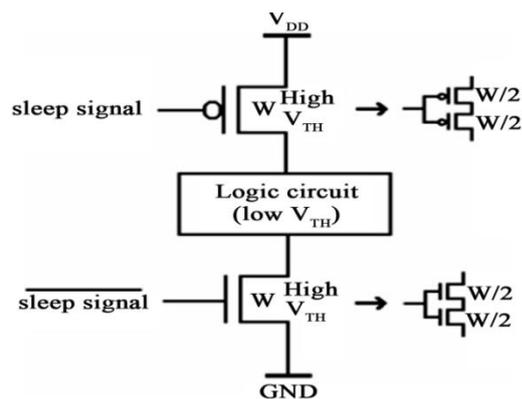
**Fig 3 Logic circuit using hybrid MTCMOS partial stack technique**
