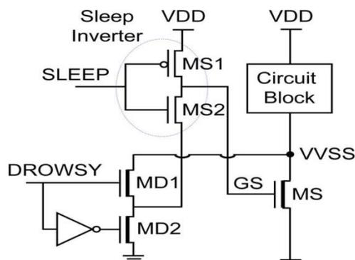
Fig 1. Implementation of the trimode footer cell.
