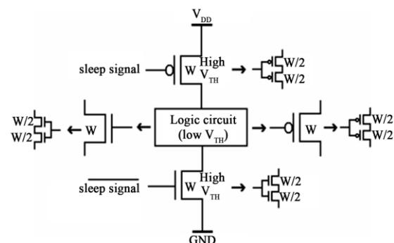
FIG 2 Logic circuit using hybrid MTCMOS complete stack technique
