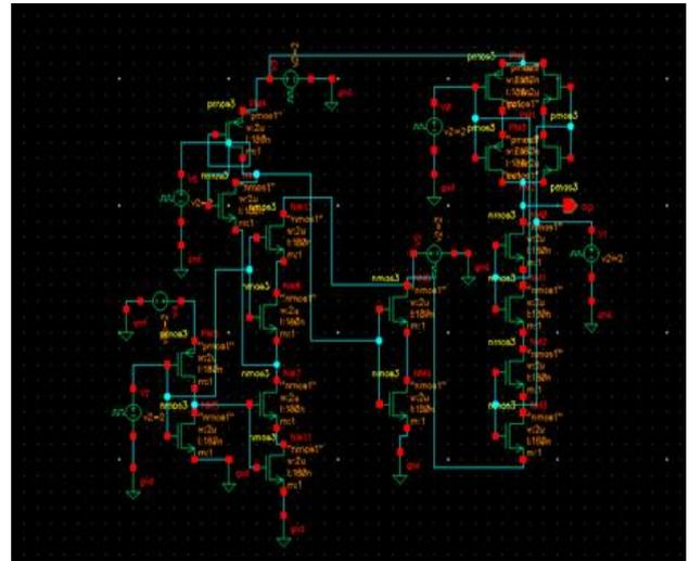
**Fig 4 Schematic Design of Hybrid MTCMOS Complete Stack Technique using tri-modal switch**
