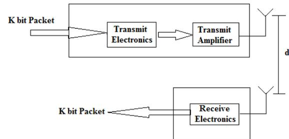
The Radio energy used in this model is same as used in [3] block diagram is presented in Fig-II, which uses a 914 MHz radio. The node radio energy consumed in transmission is given by:
