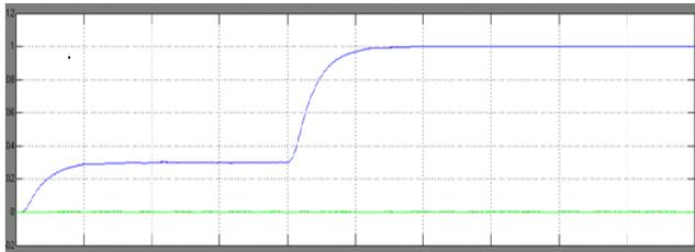
Fig.14 GRID ACTIVE AND REACTIVE POWER
