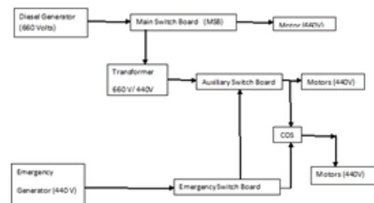
Fig.1 Block diagram of ship electrical circuit
