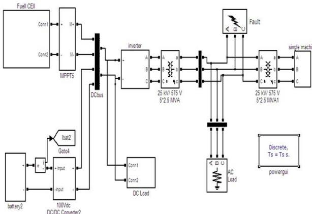
Fig.3 Simulation diagram of FCPS
