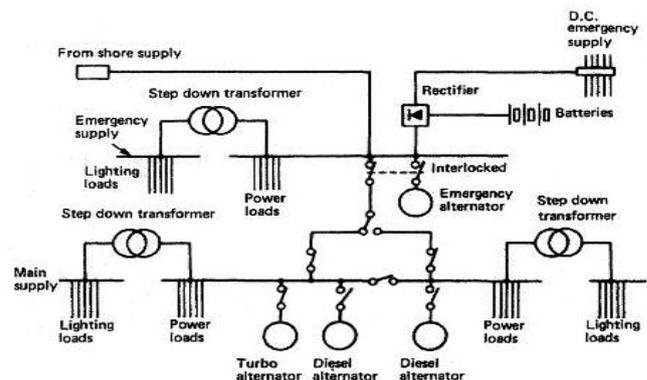
Fig. 2 On board ship electrical system power circuit
