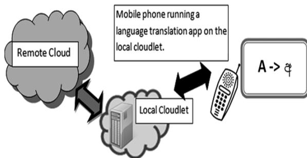
**Fig 3: A cloudlet enabling mobile devices to bypass latency and bandwidth issues while benefitting from its resources.**
