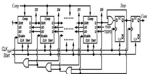
Fig.3.3. 6-bit MSAR circuit
