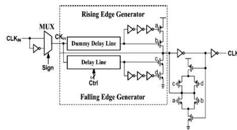
Fig.3.1. Duty cycle adjuster
