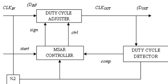
Fig.2.1. Block Diagram of the Proposed MSAR-DCC
