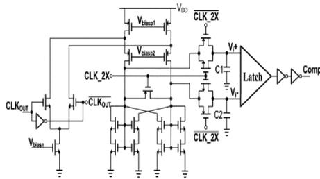
Fig.3.2. Duty cycle detector
