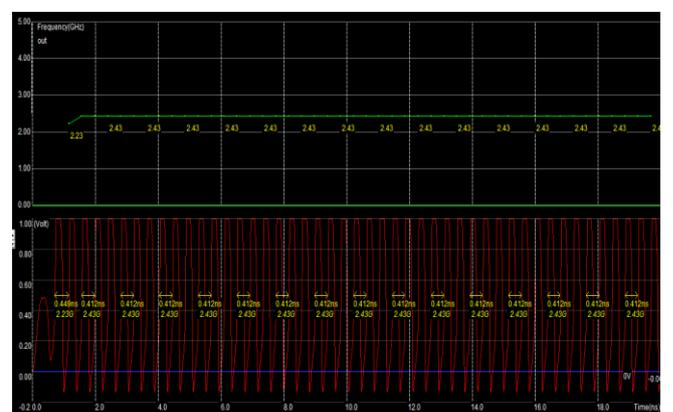
Fig.9 Layout simulation of differential LC oscillator in 90nm technology
