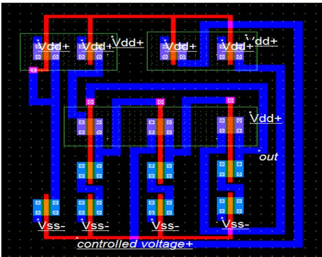
Fig.5 The layout implementation of a voltage controlled oscillator
