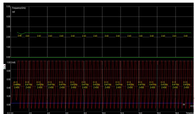
Fig.7 Layout simulation of differential LC oscillator in 120nm technology.
