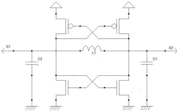
Fig.1 A differential LC oscillator
