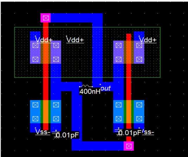
Fig.2 The layout implementation of a differential LC oscillator in 120nm technology
