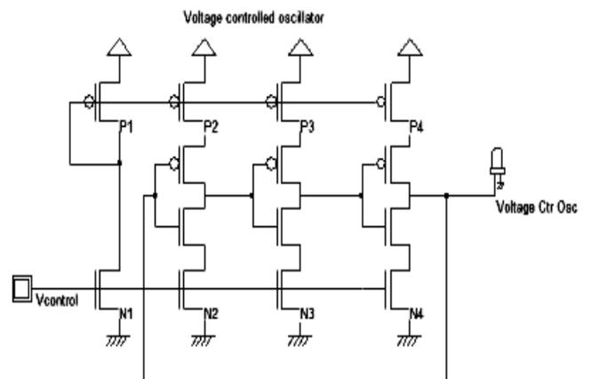
Fig.4 A voltage controlled oscillator
