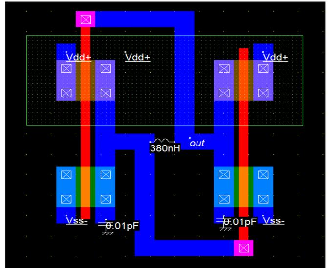
Fig.3 The layout implementation of a differential LC oscillator in 90nm technology
