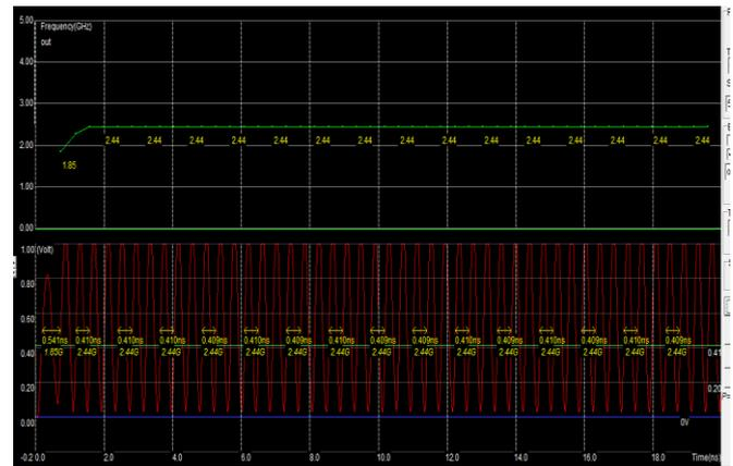
Fig.6 Layout simulation of VCO in 120nm technology.
