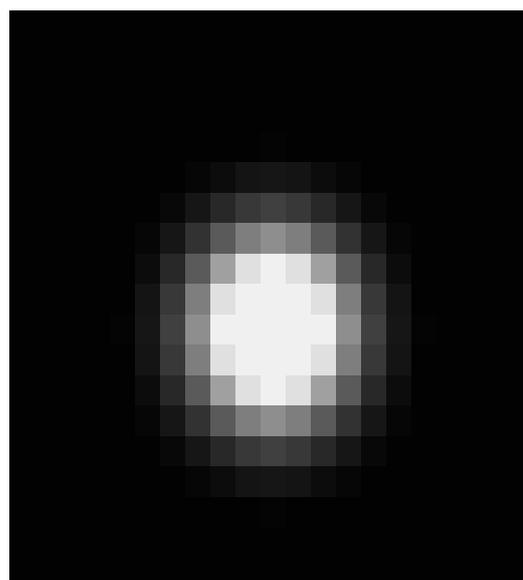
Fig1: Visual representation of a Gaussian point-spread function, left: as a 3-d surface, right: as an image
