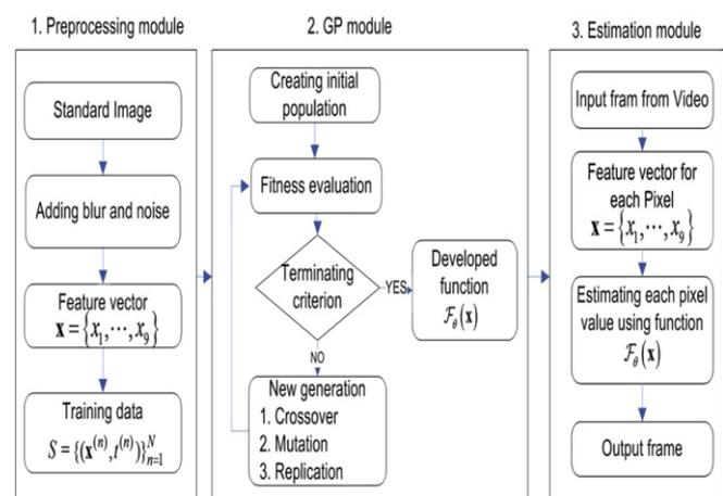
Fig. 3. Block diagram of GP
