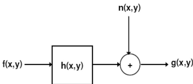
Fig:2: Degradation model
