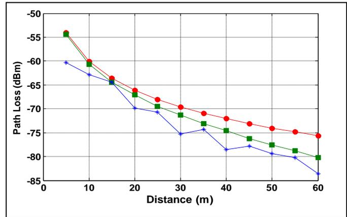
Fig.3.Path loss Comparison among Free Space and measured results
