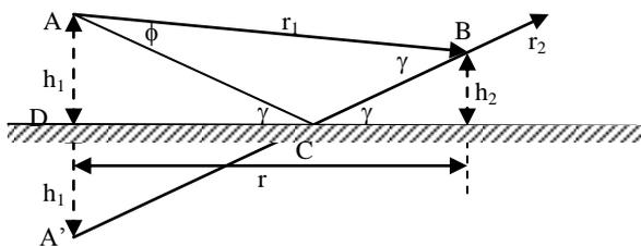
Fig. 1 Two Ray Dual Slope Model
