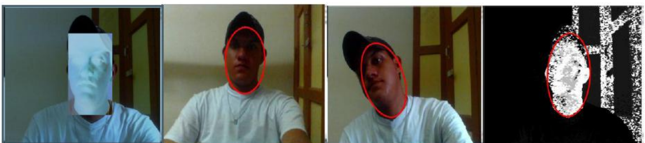
Fig 3. Tracking object using a Cam shift in sequence of frame.
