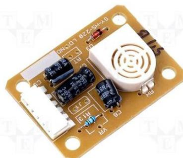
Fig. 3: Humidity Sensor Module
