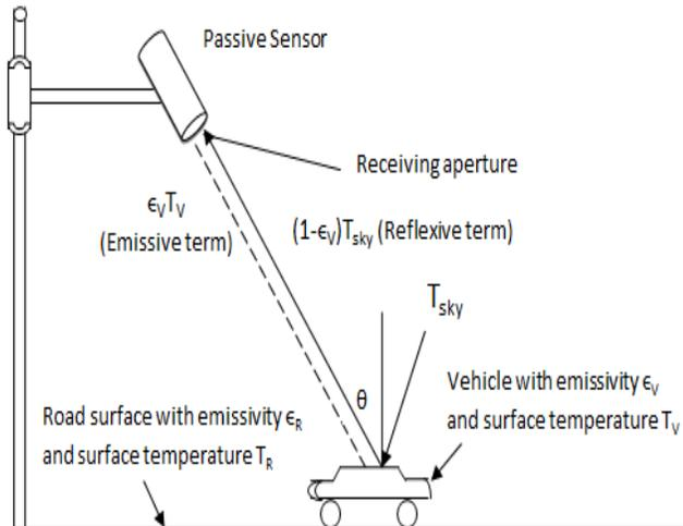
Fig. 2: Passive Infrared Sensors
