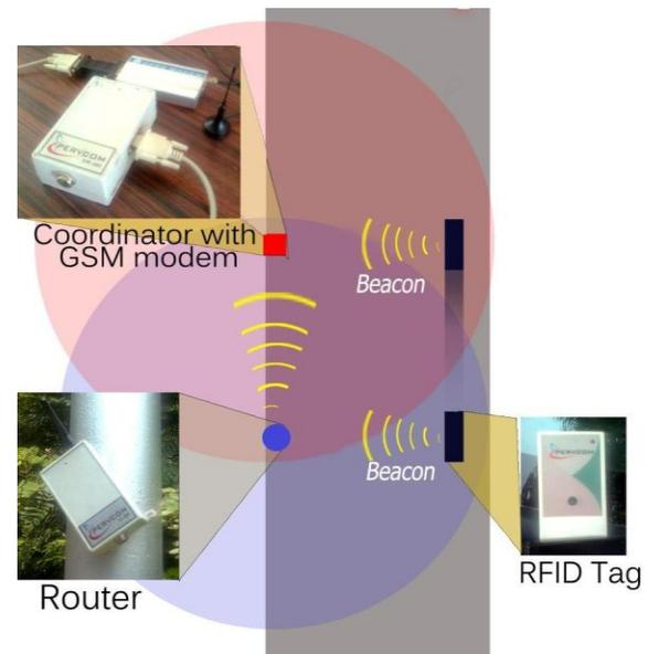
Fig.5: Working of Coordinator and Router
