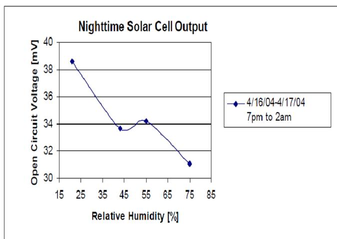
Fig.5 Open Circuit Voltage Output Of Solar Cell With Relative Humidity Conditions. [6]
