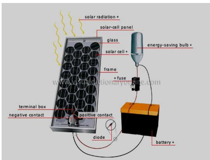
Fig.1. Basic Arrangement Of Solar Cell
