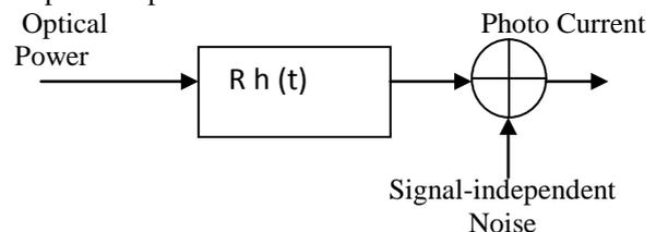
**Fig 7 Equivalent baseband model of optical wireless system using IM/DD**
