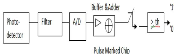
**Figure 6 Digital structure of wireless OCDMA receiver-Correlator**
