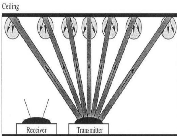
**Fig 5 A quasi-diffuse wireless optical communication system.**
