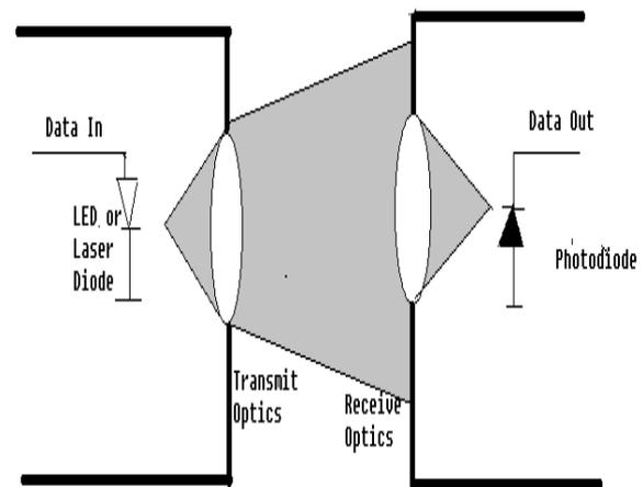
**Fig 3 Point-to-Point wireless optical communication system**
