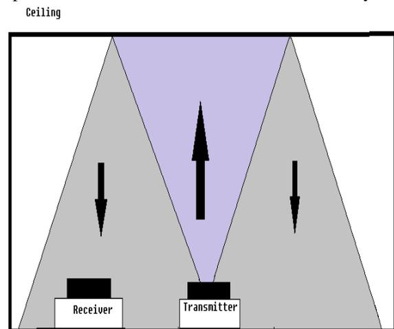
**Fig 4 A diffuse wireless optical communication system**
