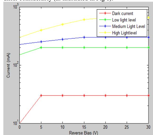
**Figure 2: Current –voltage characteristics of a photodiode**
