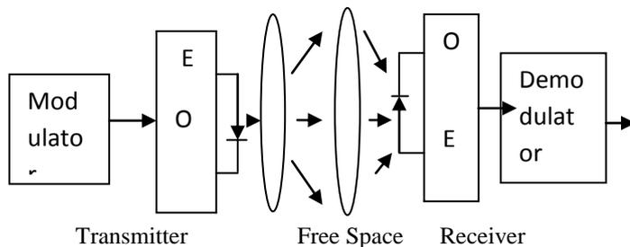
**Figure 1 Basic Optical Wireless Communication Systems**
