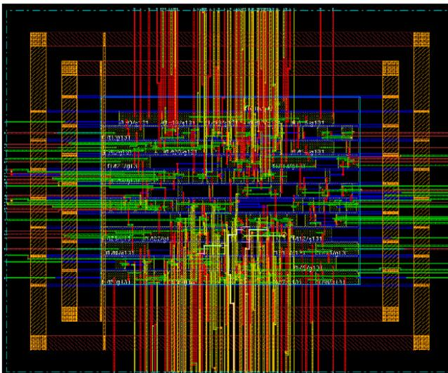
Figure 10: Layout Design of 64-bit ETA
