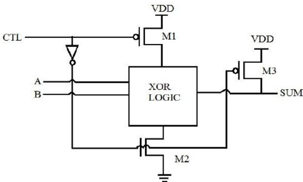
Figure 6: Schematic diagram of XOR gate
