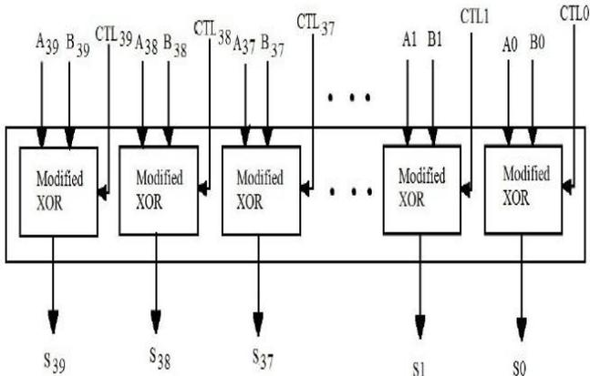
Figure 5: Architecture of Carry Free Addition Block
