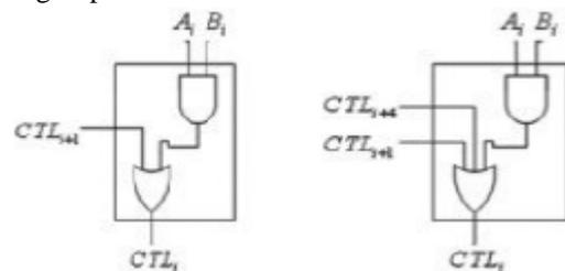
Figure 4: Control signal generating cells of type I & II
