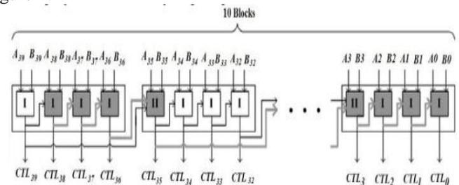
Figure 3: Control Block for first 40 bits
