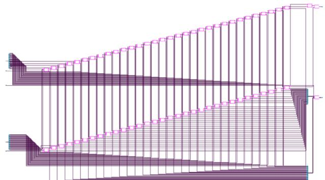
Figure 8: Schematic circuit of carry select adder
