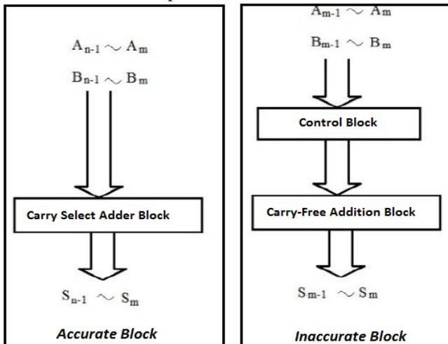
Figure 2: Hardware Implementation of Proposed Adder
