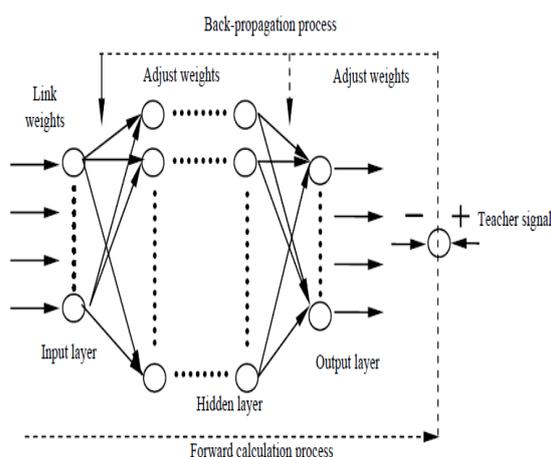
Figure 4. The structure of BP neural network
