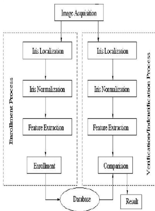
Fig 1. Block diagram of an iris recognition system
