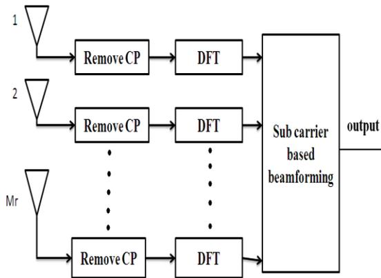
Fig. 2. Receive Beamforming
