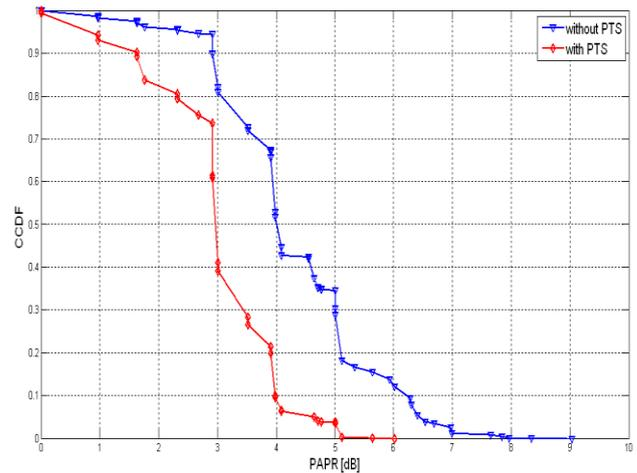
Fig.8 Comparison of PAPR with PTS technique and without PTS technique
