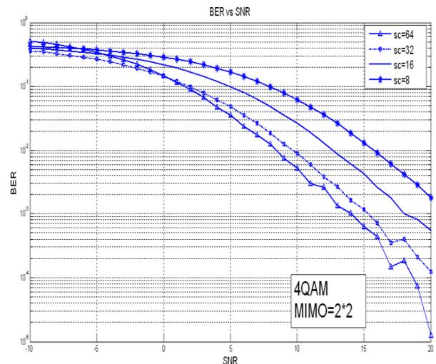
Fig.6 BER vs. SNR for 4-QAM for various subcarrier with dimensions of MIMO as 2x2
