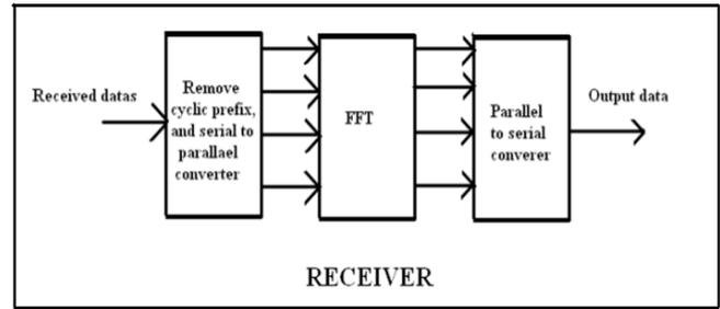
Fig.3 Cognitive radio receiver with OFDM
