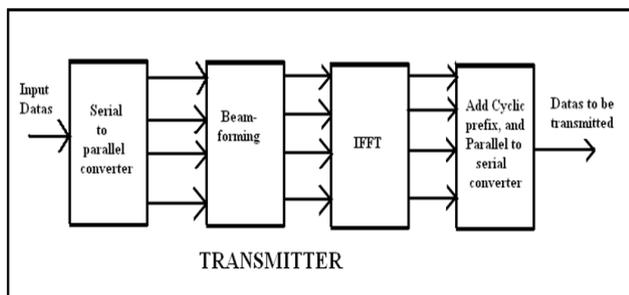
Fig.2 Cognitive radio transmitter with OFDM
