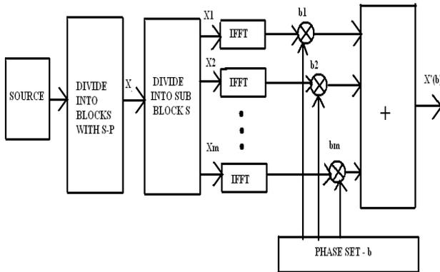
Fig.4 Block Diagram of PTS
