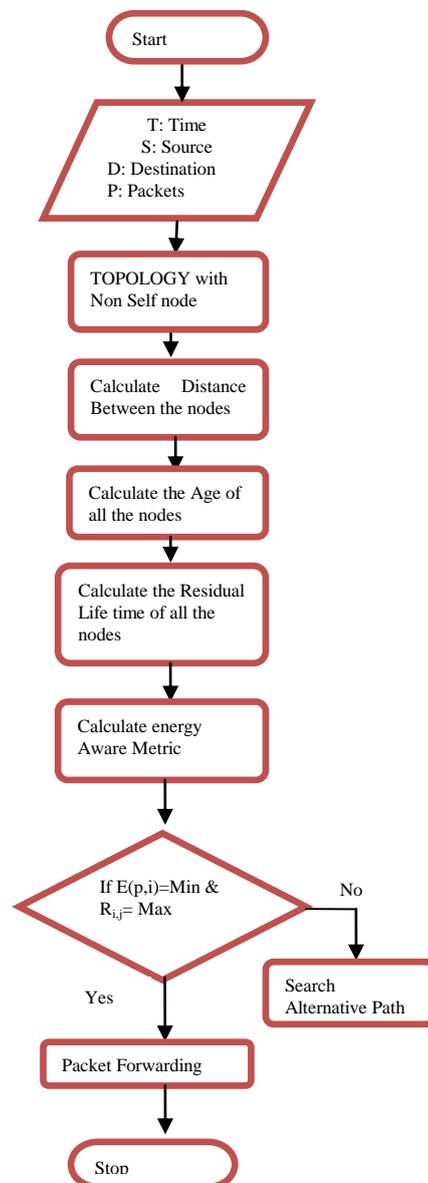
Fig: 5. System Flow Diagram for Routing
