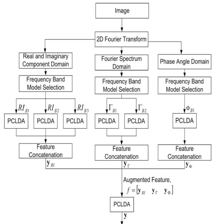
Fig.5. Structure of fourier feature
