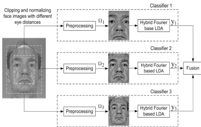
Fig.6. Structure of Fourier-based LDA with multiple face models.
