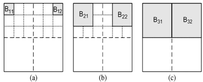
Fig. 4. Feature regions are selected according to different frequency bands in Fourier features. The upper left point of all quadrangles (0, 0) is the lowest frequency, and notations are  $B_1, B_2$ , and  $B_3$ .
