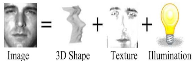
Fig. 2. Under the assumption of the Lambertian reflectance model, an image consists of a 3-D shape, texture, and illumination.
