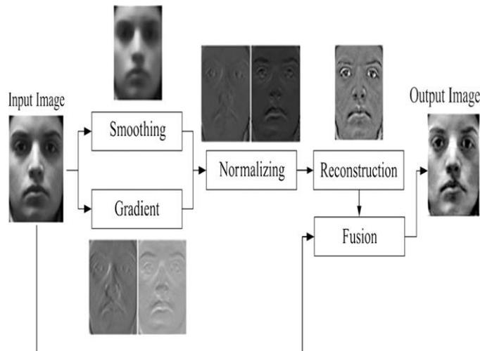
Fig.3. Structure of the integral normalized gradient image
