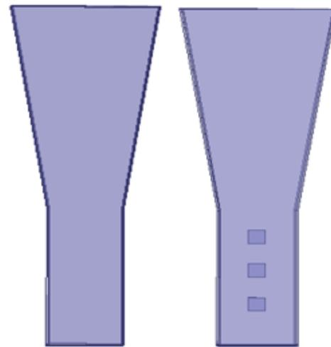
Figure [1]. A) H-plane Horn Antenna B) H-plane Horn Antenna with two EBG unit cells inside the wave Guide
