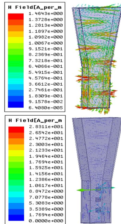
Figure [8]. H- field analysis comparison for antenna without and with EBG
