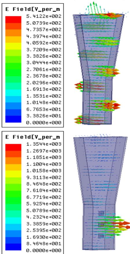
Figure [7]. E- field analysis comparison for antenna without and with EBG
