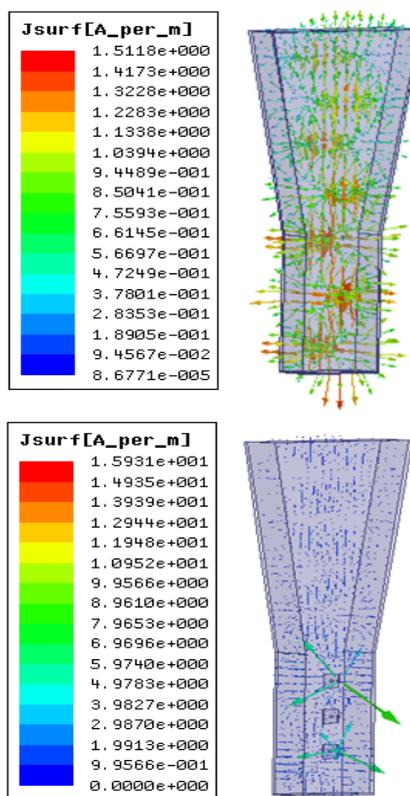
Figure [9]. H- field analysis comparison for antenna without and with EBG
