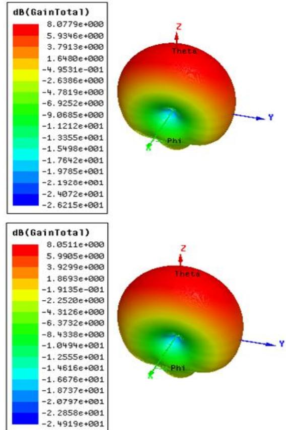
Figure [5]. Gain in 3D curves A) H-plane Horn Antenna B) H-plane Horn Antenna with two EBG unit cells inside the wave Guide
