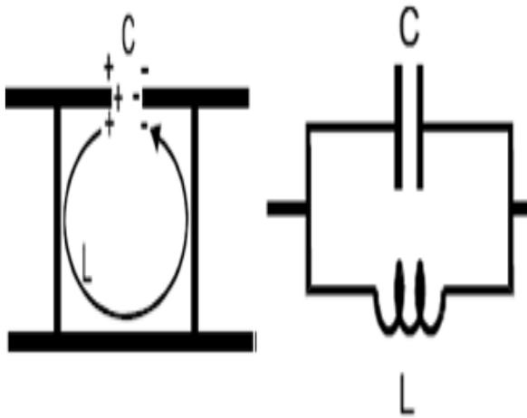
Fig [2] EBG Unit cell, its equivalent
