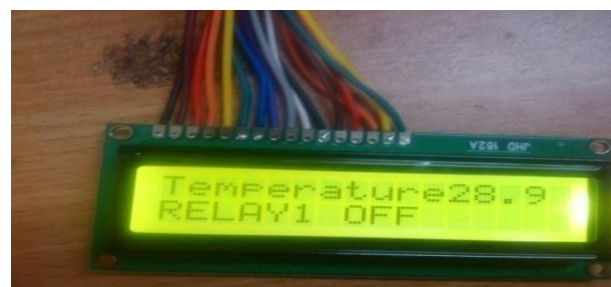
Snap 1:-Temperature measurement on LCD display
