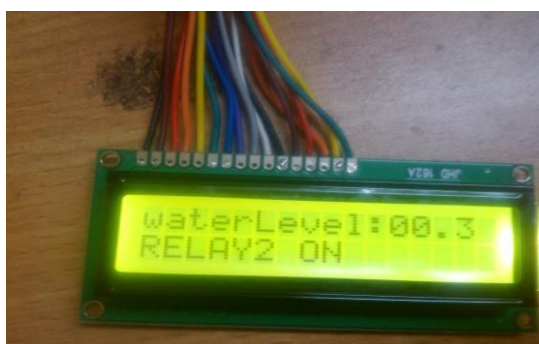
Snap 5:-Water Level reading on LCD display
