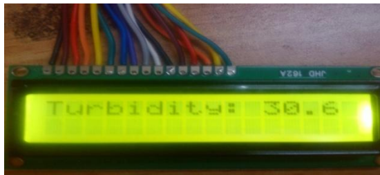
Snap3:-Turbidity measurement on LCD display
