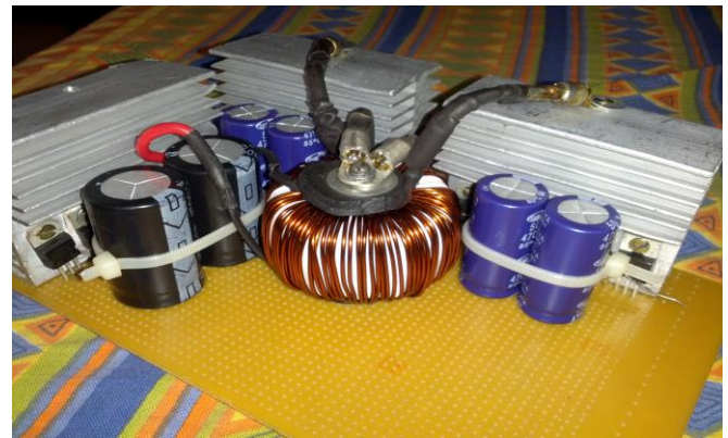
Fig. 8 Prototype of isolated buck-boost Converter
