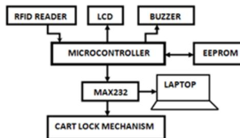
Fig.1 Block Diagram of Smart Cart
