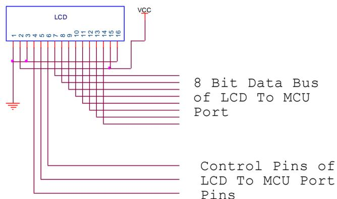
Fig.4 Pin Configuration of LCD
