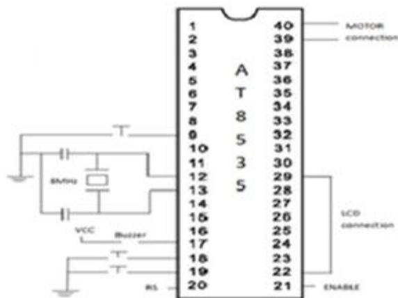
Fig.2 Interfacing of Microcontroller
