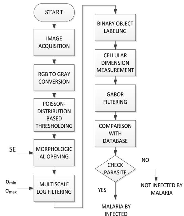
Fig. 2 Flow chart outlining the main steps of the proposed system.
