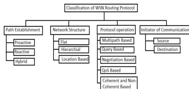
Fig1 Classification of Routing Protocols in Wireless Sensor Network.
