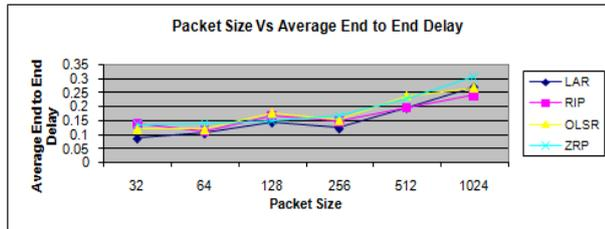
Fig. 10. Average End to End Delay analysis of 60 nodes in Physical Layer for different Routing Protocols
