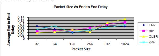
Fig. 6. Average End to End Delay analysis of 20 nodes in Physical Layer for different Routing Protocols
