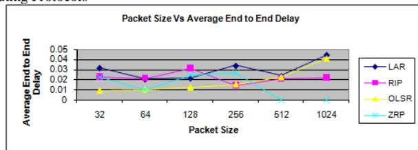
Fig. 5. Average End to End Delay analysis of 10 nodes in Physical Layer for different Routing Protocols
