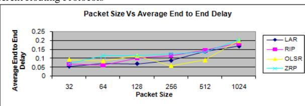
Fig. 8. Average End to End Delay analysis of 40 nodes in Physical Layer for different Routing Protocols
