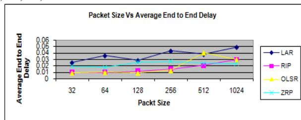
Fig. 4. Average End to End Delay of 5 nodes in Physical Layer for different Routing Protocols
