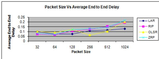
Fig. 9. Average End to End Delay analysis of 50 nodes in Physical Layer for different Routing Protocols
