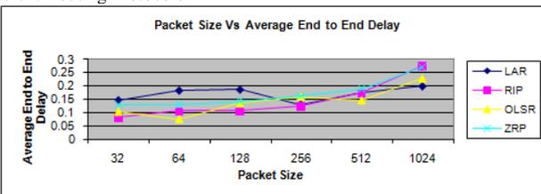
Fig. 7. Average End to End Delay analysis of 30 nodes in Physical Layer for different Routing Protocols
