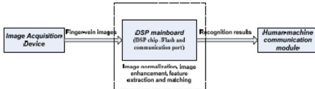
Fig. 1. The hardware configuration of the FVAS
