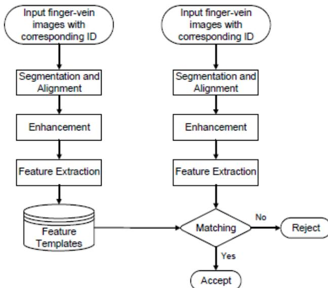
Fig. 2. The flowchart for the FVAS algorithm
