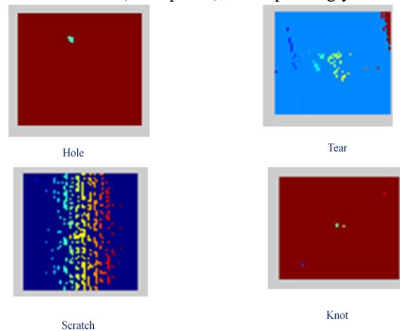
Fig.9 Graph Based Segmentation of Hole,Tear,Scratch & Knot
