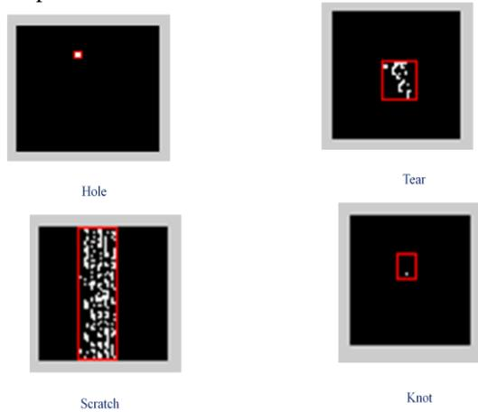
Fig.10 Recognition of Hole, Tear, Scratch & Knot
