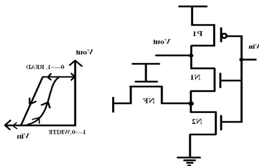
Fig.3.1 Conceptual ST schematics, the gate connection of the feedback transistor is connected to the  $V_{cc}$  to show the feedback mechanism during 0->1 input transition.
