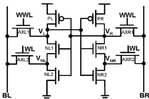
Fig.3.5 ST-2 bit cell
