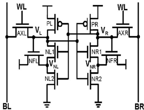
Fig.3.4 ST-1 bit cell
