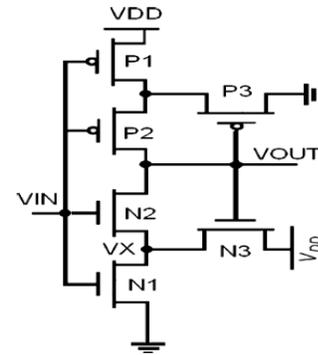
Fig.3.2.Implementation of a Schmitt trigger
