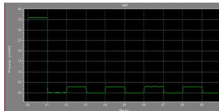
Fig.7.8 Power Consumption Profile For 8T ST Bit cell operation
