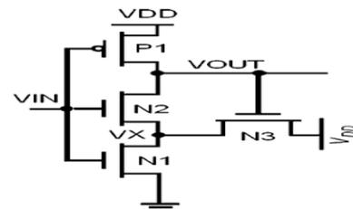
Fig.3.3 Modified Schmitt Trigger
