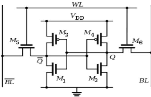
Fig.2.1 CMOS six transistor SRAM cell
