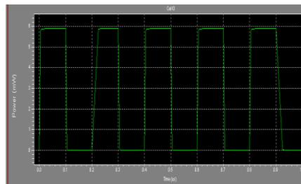
Fig.7.6 Power Consumption Profile For ST1 operation
