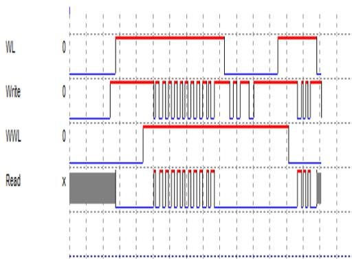
Fig.7.2 Circuit and simulation waveforms for ST1 operation
