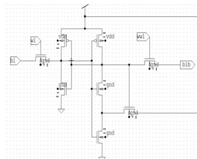
Fig.5.1 Proposed 8T ST Bit cell
