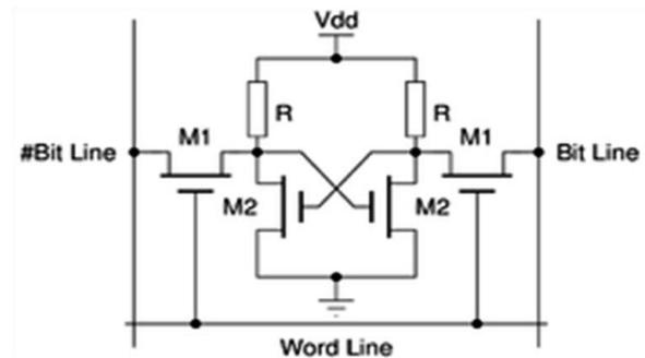
Fig.2.2 A four transistor SRAM cell
