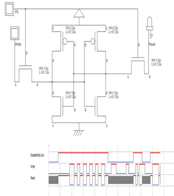
Fig.7.1 Circuit and simulation waveforms for 6T operation
