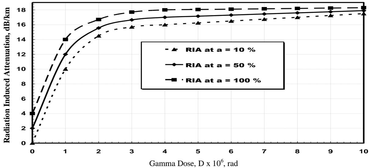
Fig.3. Variations of the attenuation against gamma dose as a function of probability of defect generation (a) with operating wavelength = 850 nm and dose rate = 0.1 (krad/min).
