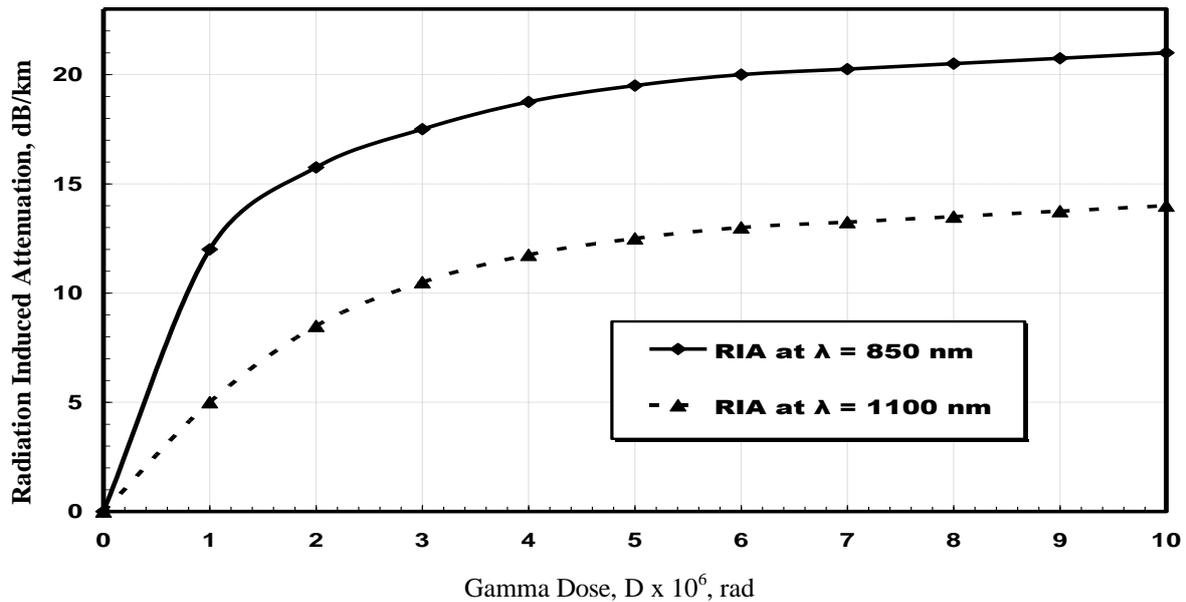
Fig.5. Variations of the attenuation against gamma dose as a function of operating wavelength ( $\lambda$ ) with dose rate = 0.1 (krad/min) and probability of defect generation ( $\alpha$ ) = 100%.
