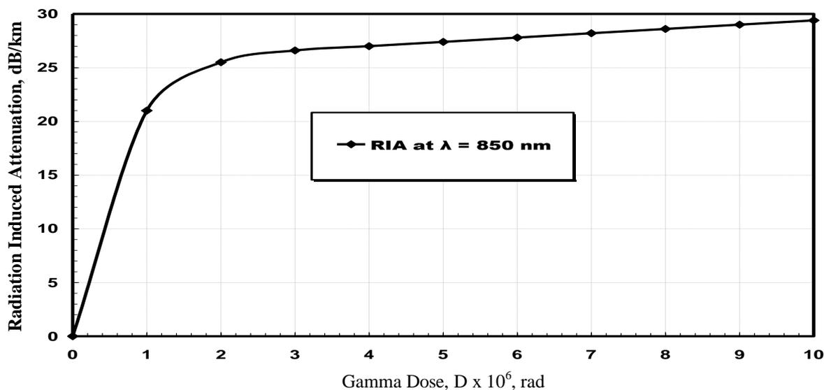
Fig.2. Variations of the attenuation against gamma dose with operating wavelength= 850 nm, dose rate =0.1 (krad/min) and probability of defect generation = 100%.
