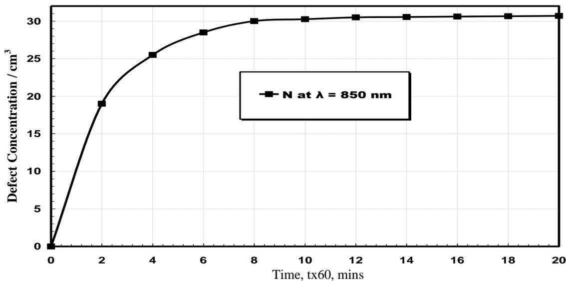
Fig.7. Variations of the attenuation against time with operating wavelength= 850 nm, dose rate = 100 krad/min, radiation dose = 1 Mrad and probability of defect generation = 100%.
