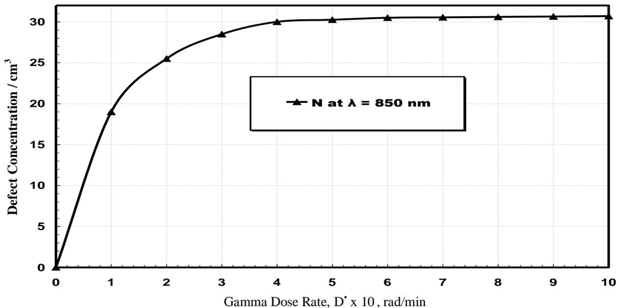
Fig.6. Variations of defect concentration against the gamma dose rate with operating wavelength= 850 nm, radiation dose = 1 Mrad and probability of defect generation = 100%.
