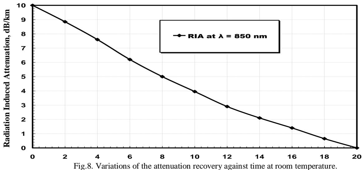
Fig.8. Variations of the attenuation recovery against time at room temperature.
