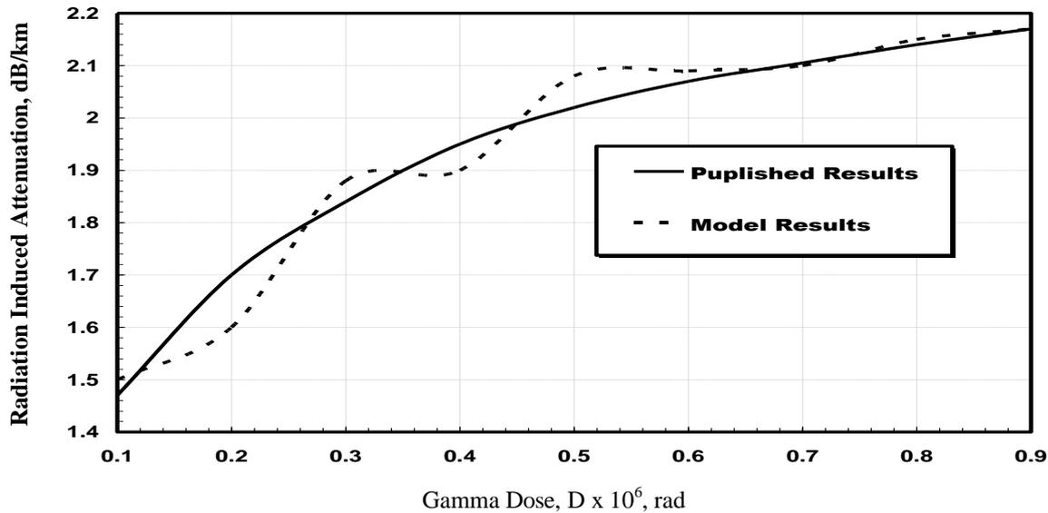
Fig.1. Variations of the radiation induced attenuation against gamma dose with operating wavelength= 850 nm and dose rate =0.1 krad/min.
