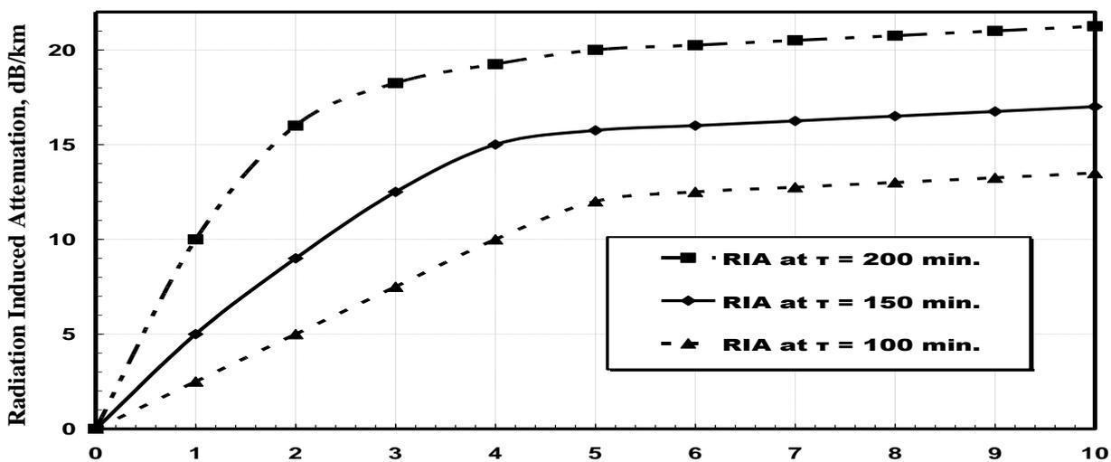
Fig.4. Variations of the attenuation against gamma dose as a function of characteristic lifetime of the defect (τ) with operating wavelength= 850 nm, dose rate=0.1 (krad/min) and probability of defect generation (a) = 100%.
