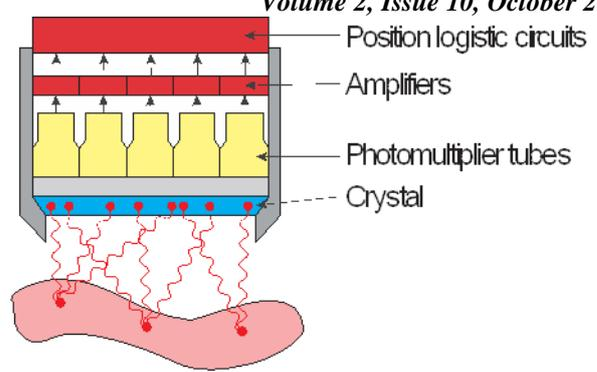
Figure 5 – Gamma camera construction (without collimator)
