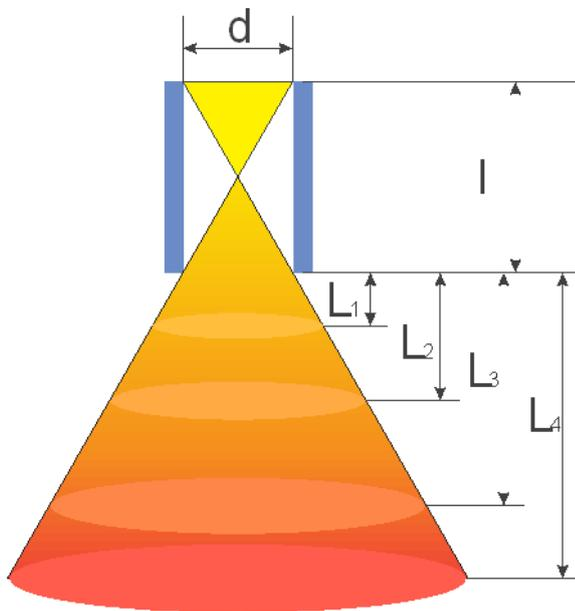
Figure 8 – Readable area dependent on hole deep and diameter, and distance object from collimator
