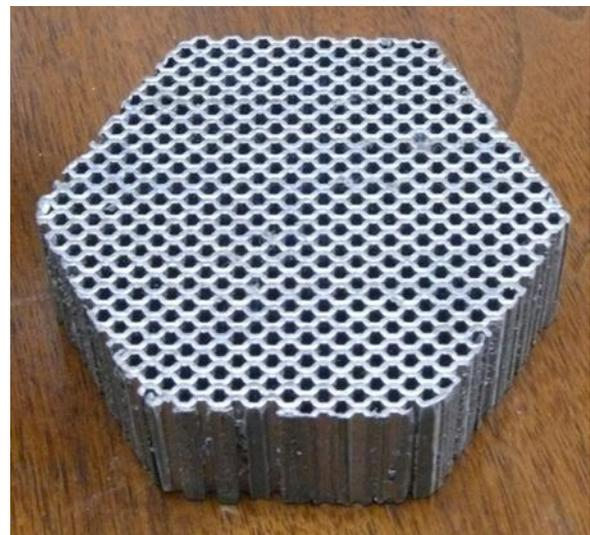
Figure 6 – Part of parallel collimator
