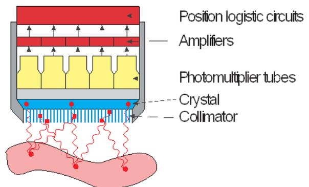
Figure 7 – Gamma camera construction (with collimator)
