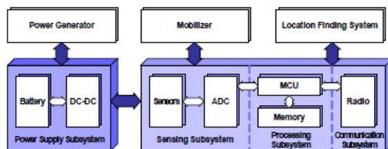
FIG. 3: Architecture of a typical wireless sensor node.
