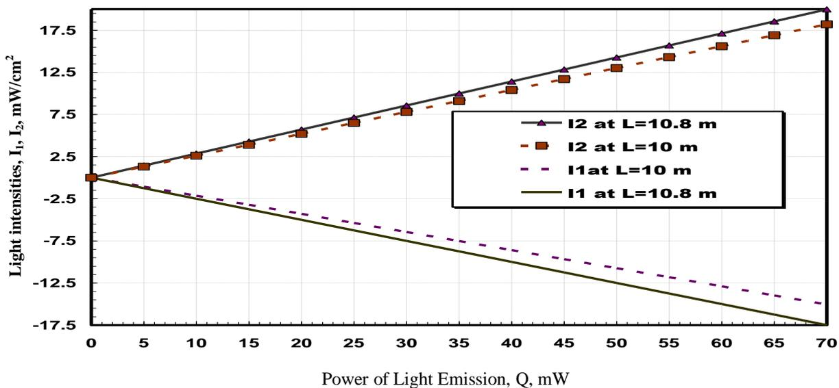
Fig.6. Variations of the light intensities ( $I_1, I_2$ ) against light emission power (Q) at different optical fiber lengths (L).
