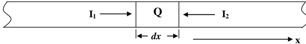
Fig.1. Optical fiber in which the light is propagating in x direction.
