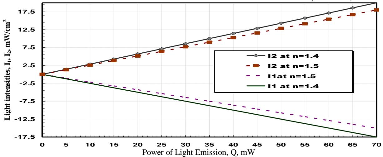
Fig.7. Variations of the light intensities ( $I_1, I_2$ ) against power of light emission ( $Q$ ) at different refractive indices ( $n$ )
