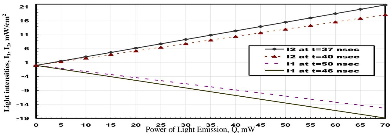
Fig.9. Variations of the light intensities ( $I_1, I_2$ ) against power of light emission ( $Q$ ) at different emission light traveling times ( $t$ )
