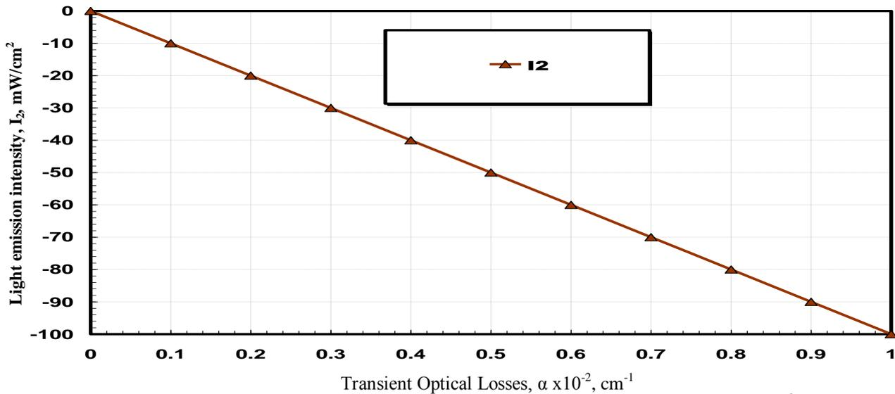
Fig.5. Variations of the light emission intensity ( $I_2$ ) against the transient optical losses  $\alpha$  with  $V_1=2 \times 10^8$  m/sec,  $V_2=2.5 \times 10^8$  m/sec, and  $k=0.1$
