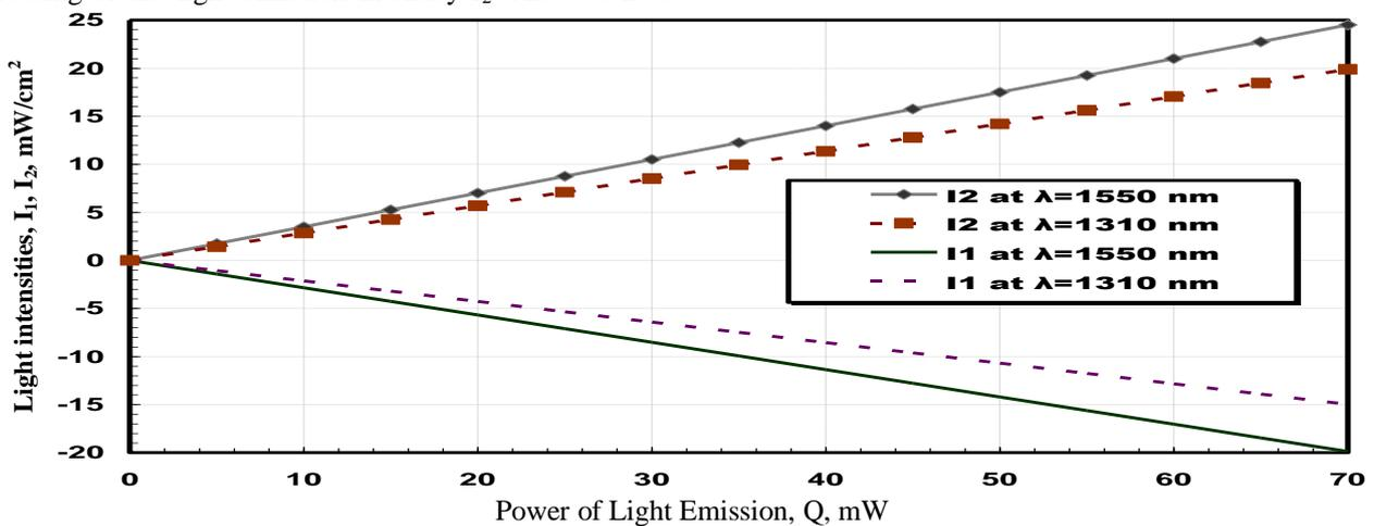
Fig.8. Variations of the light intensities ( $I_1, I_2$ ) against power of light emission ( $Q$ ) at different operating wavelengths ( $\lambda$ )
