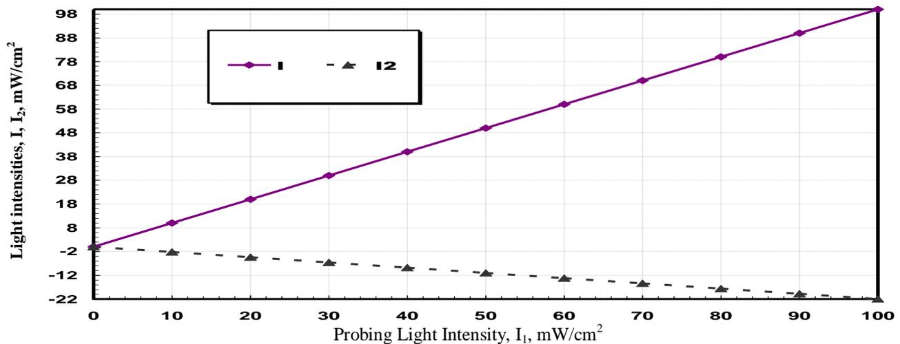
Fig.3. Variations of the probing light intensity ( $I_1$ ) against propagating light intensity ( $I$ ) and light emission intensity ( $I_2$ )
