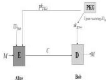
Fig:5 identity based encryption
