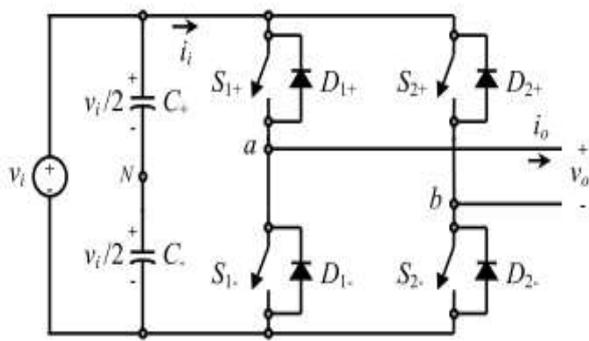
Fig. I: Voltage Source Inverter.
