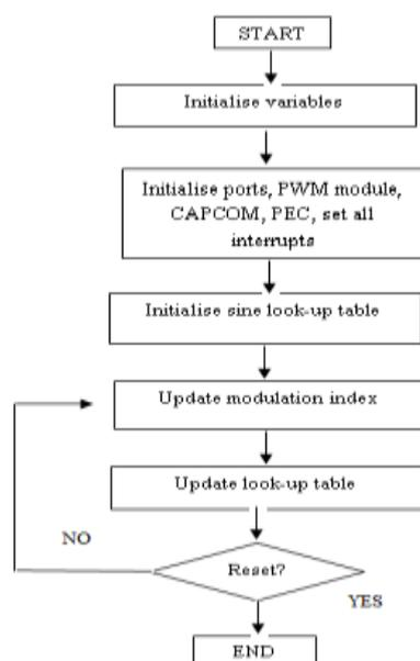
Figure 3. Flow-Chart for the PWM generation
