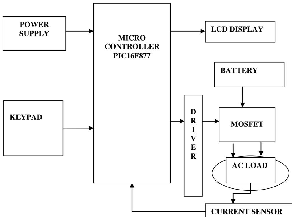
Fig. II: Proposed System of PWM inverter
