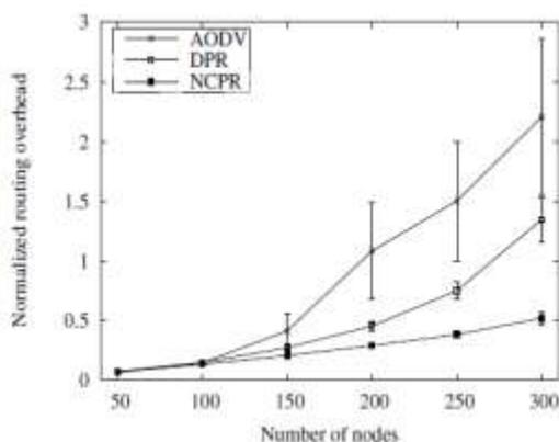
**Fig. 2. Normalized Routing Overhead With Varied Number Of Nodes**
