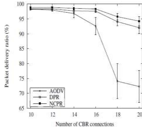
Fig. 7. Packet Delivery Ratio With Varied Number Of CBR Connections
