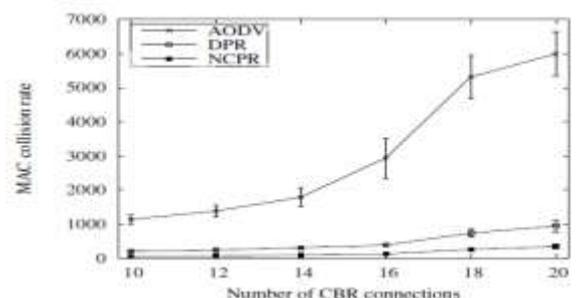
**Fig. 5. MAC Collision Rate With Varied Number Of CBR connections**
