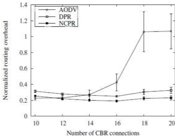
Fig. 6. Normalized Routing Overhead With Varied Number Of CBR Connection
