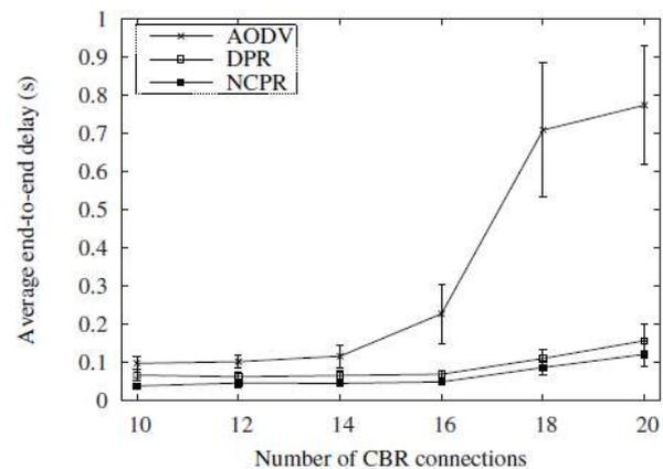
Fig. 8. Average end-to-end Delay With Varied Number Of CBR Connections
