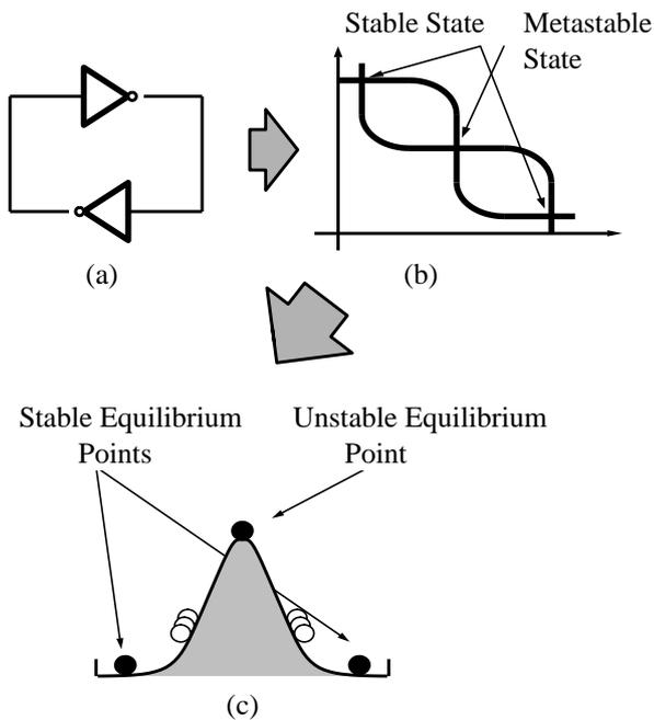
Figure 1: Mechanical analogy for metastable state. (a) Regenerative circuit; (b) load line representation; (c) mechanical analogy
