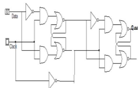
Figure 2(a): Delay Latch using cross coupled NAND gates
