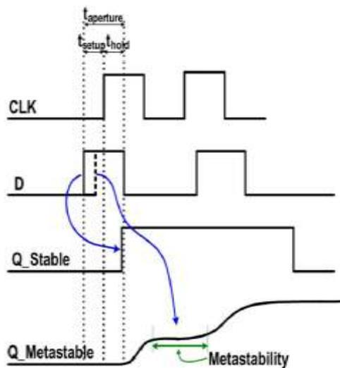
Figure 2(b): Flip-Flop waveforms in case of stable and metastable output
