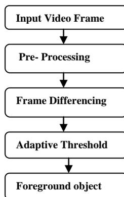
Fig. 1 Block Diagram of FD Background Subtraction Method with Post- Processing
