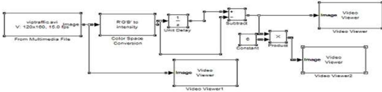
Fig.2 Simulinks model for frame differencing technique
