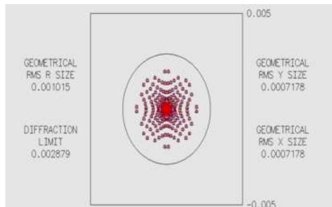
**Fig: 3. Spot diagram of pre-collimation cylinder**
