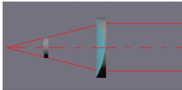
**Fig: 2. Pre-collimation cylinder lenses system**
