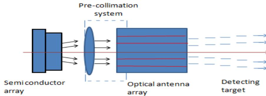
**Fig: 1. Emitting optical system structure**
