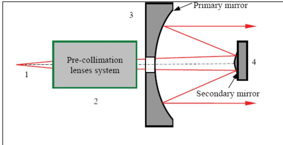
Fig. 6. One unit optical system structure
