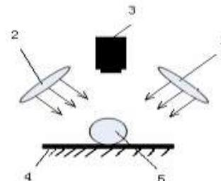
Figure 4: Fruit system light and camera location. 1-light; 2-light; 3-cmos camera; 4-conveyor belt; 5-fruit
