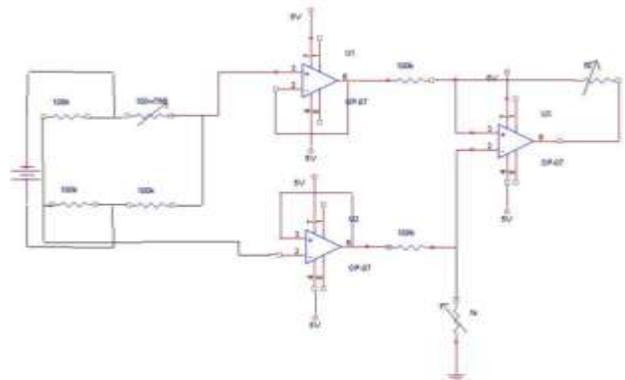
Figure 9: Load cell circuit arrangement
