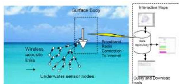
Fig 1. An example scenario for underwater sensor networks
