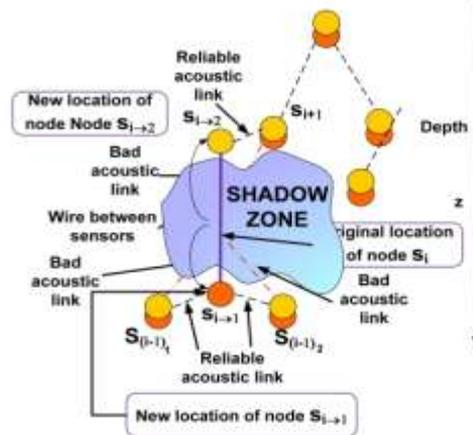
Fig 4. Nodes placed in bad acoustic links
