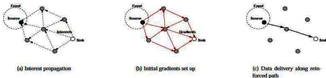
Fig1. A Simplified Schematic for directed diffusion
