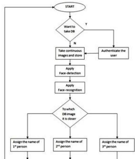
Figure5. Overall flow chart of the software
