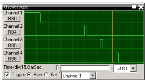
Fig.7(b) Triggering pulses on Real PIC Simulator
