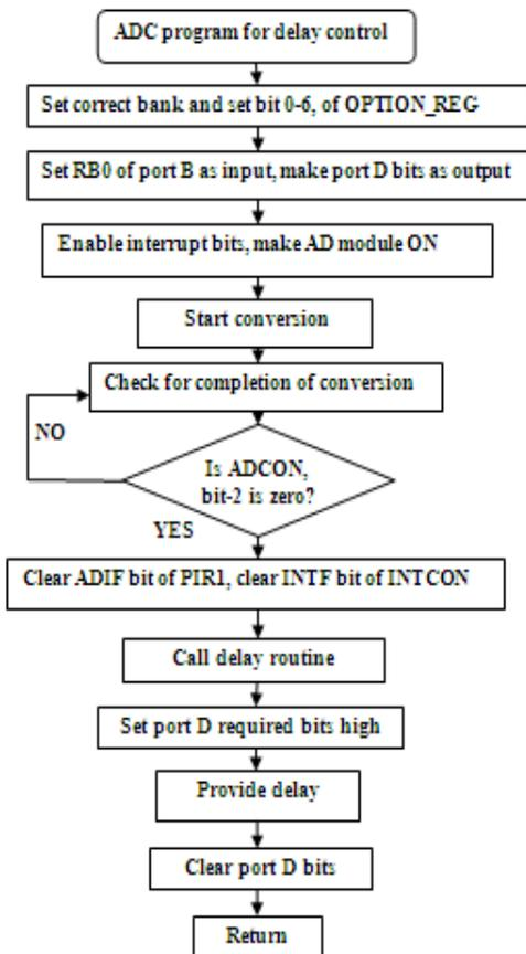
Fig.4 Flowchart of ADC program for delay control
