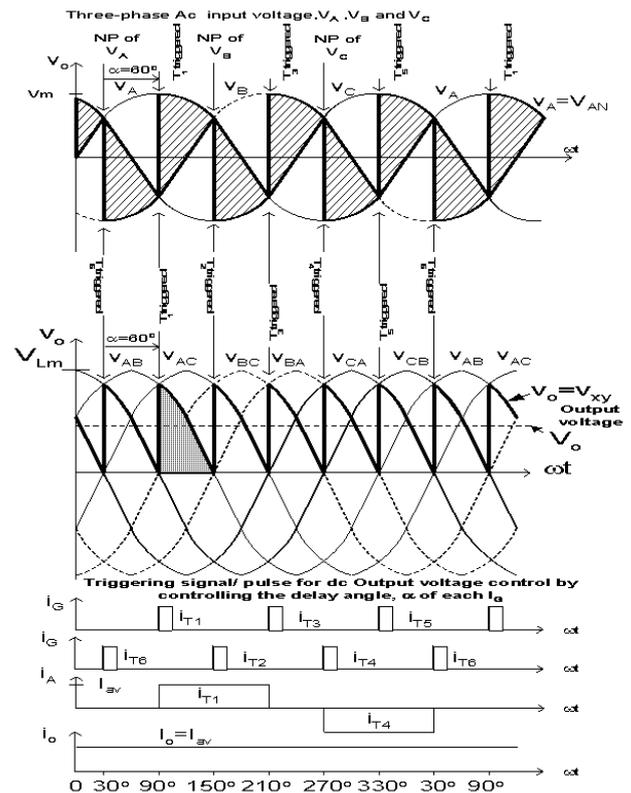
**Fig.2 Triggering signal/pulse for dc output voltage.**
