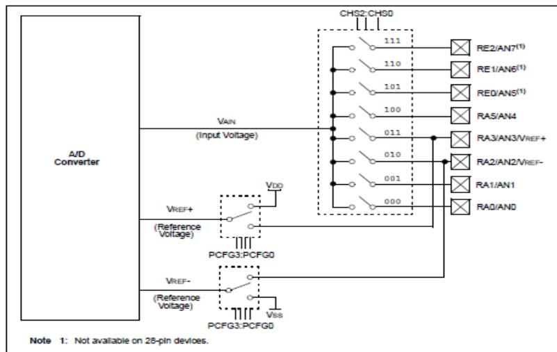
Fig. 6 A/D Block Diagram
