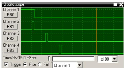
Fig.7(a) Triggering pulses on Real PIC Simulator
