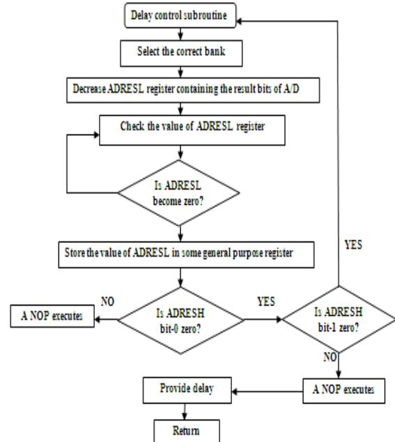
Fig.5 Flowchart for delay control subroutine
