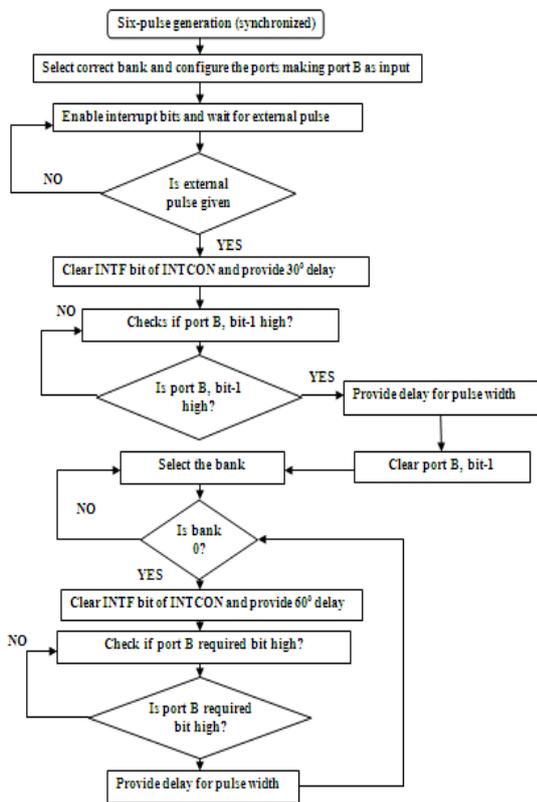
Fig.3 Flowchart for six-pulse generation
