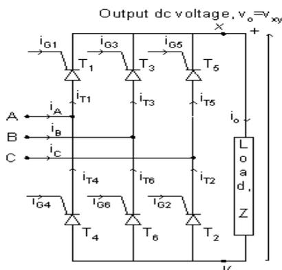
**Fig.1 Power circuit of three-phase, full-wave six-pulse, controlled ac to dc converter.**
